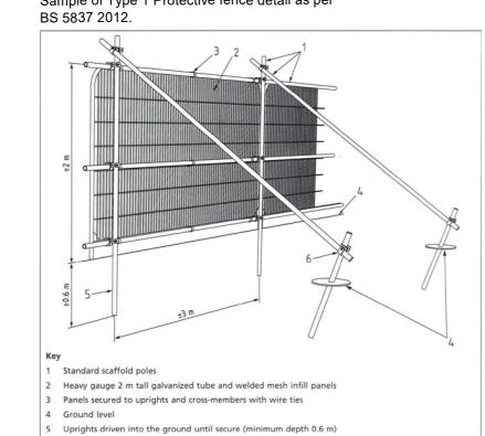
The tree protection fencing is to be erected enclosing the root protection areas around the trees being retained as shown on this drawing and appendix 1\_In some areas, the site hoarding may be sufficient to act as the protective fencing if the tree and its root zone are positioned outside and no works are envisaged within the area outside the site hoarding. This will need to be discussed and agreed at the initial site meeting.
