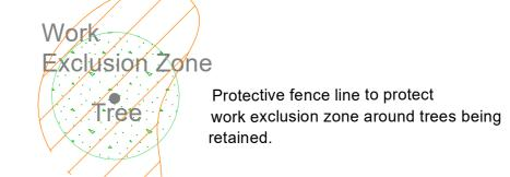
Sample of Type 1 Protective fence detail as per
